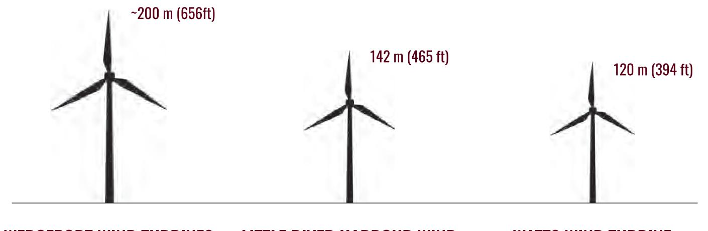
Wedgeport Wind turbines are 30% taller than Little River Harbour Wind and 40% taller than Watts Wind, but produce 3 to 4x more power per turbine. This results in fewer turbines being needed to deliver the Project's energy generation capacity.
